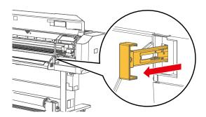
Pull the media toward the front and use a personal cutter to cut the torn part of the media along the groove.
