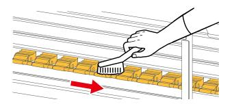
Using a paper towel or soft cloth dampened with in a small amount of ethanol, clean the platen, media guide and edge holders to remove dust.
