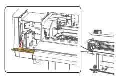
Look at the bottom surface of the UV-LED lamp and wipe off any sticking ink or dust with a paper towel.
