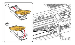
Fill 30 ml of maintenance cleaner into the flushing box.
