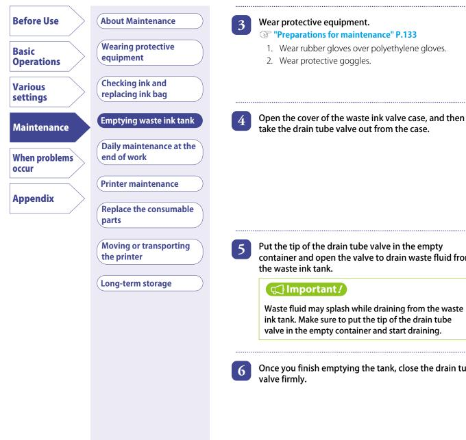
Put the tip of the drain tube valve in the empty container and open the valve to drain waste fluid from the waste ink tank.
