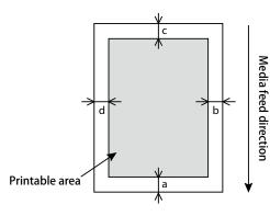
a=5 mm \*1 b=5 mm to 25 mm \*2 c=5 mm d=5 mm to 25 mm \*2 \*1 The margin will be 15 mm in the following cases: • The first printing after media initialization • When feeding the media backward by using ▲ key. The margin will be 40 mm in the following cases: • When the Media Initial menu is set to "Top&Width" • After cutting the media
